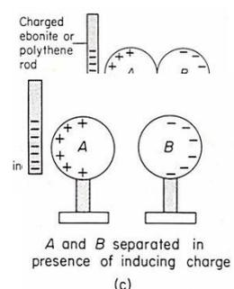
4. Now remove the negatively charged rod as well and test the charge of sphere A and B. Both will possess charge. Sphere A will be negatively charged and B will be positively charged.
