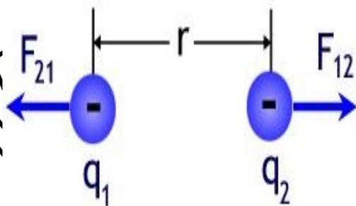
Where 'K' is constant and its value in SI unit is  $9 \times 10^9 \text{ Nm}^2/\text{C}^2$ . The constant 'K' is commonly expressed as follows.
